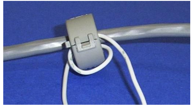
Ferrite core installation.
